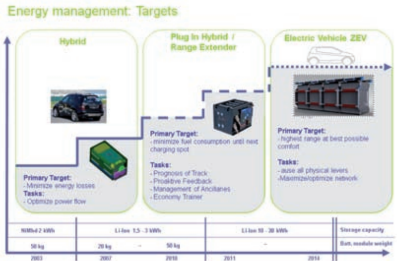
Figure 4: Electric storage dimensioning: motivation and tasks
